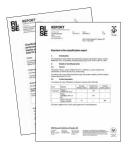
This system is **classified as B**, the highest fire-retardant rating that can be expected for an organic material like wood. In terms of smoke production, the system is rated **s2**. The fire redardant system received the best possible score, **d0**, for zero formation of burning droplets.
